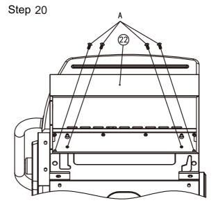
Assemble the side table (R) (22) to the firebox by hanging it to the half screwed bolts, fasten it with 4 bolts (A). Then secure the half screwed bolts.
