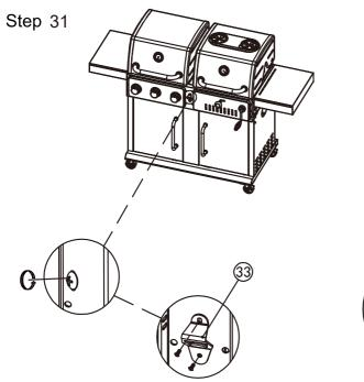
Loosen 2 bolts of the middle of control panel, fasten the bottle opener (33) to fireboxes, screw back the bolts as shown.
