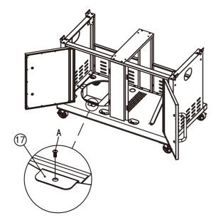
Install tank base upper (17) to the bottom shelf with 2 bolts (A).
