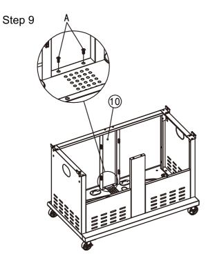
Assemble the front support (10) to bottom shelf with 2 bolts (A).
