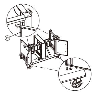
Slide the door axles (15) to doors, install them to the cart front beam and bases.
