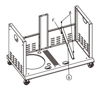
Fasten the LP barrie bar(6) to the bottom shelf with 1 bolt (A) and to the rear shelf with 1 bolt (A) and 1 nut (F).
