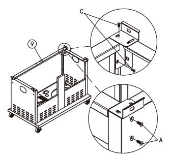
Assemble the cart front beam (9) to side shelves with 4 bolts (A) and 4 bolts (C).
