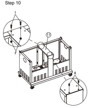
Assemble the middle brace (11) to cart front beam with 2 bolts (I) and 2 nuts (F) and to back support with 2 bolts (A).
