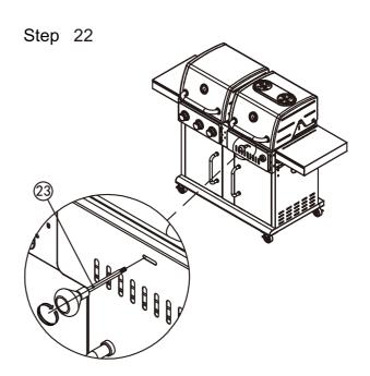
Fasten the side tables from the inside of the fireboxes with 8 bolts (A).
