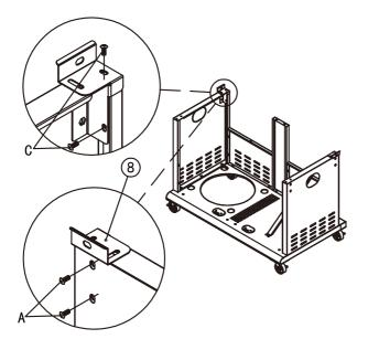
Assemble the left firebox brace (8) to the shown positions of side shelf with 2 bolts (A) and 2 bolts (C).
