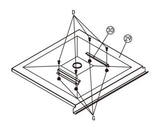
Assemble the grease cup brace (30) to the grease tray (29) with 4 bolts (D) and 4 nuts (G).
