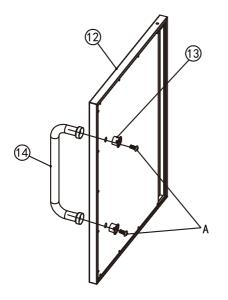
Assemble the door handles (14), handle bases (13) to the doors (12) with 4 bolts (A).
