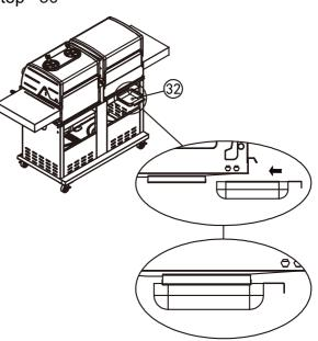
Slide the ash pan (31) and grease tray (29) underneath the fireboxes.
