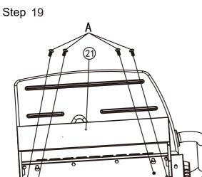
Assemble the side table (L) (21) to the firebox by hanging it to the half screwed bolts, fasten it with
